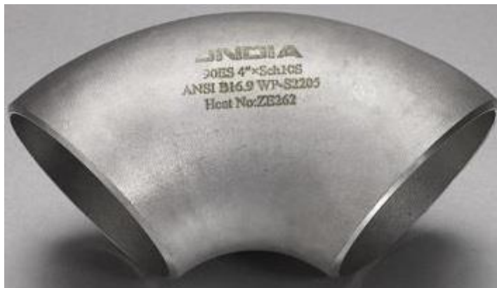
Duplex stainless steel 2205, short radius elbow 90°, 4" SCH10S, ASME B16.9
