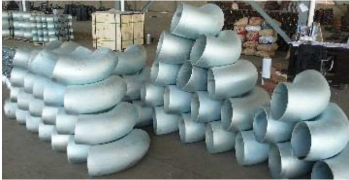
ASME B16.9 long radius elbows, 10" SCH40 90°, galvanized.
