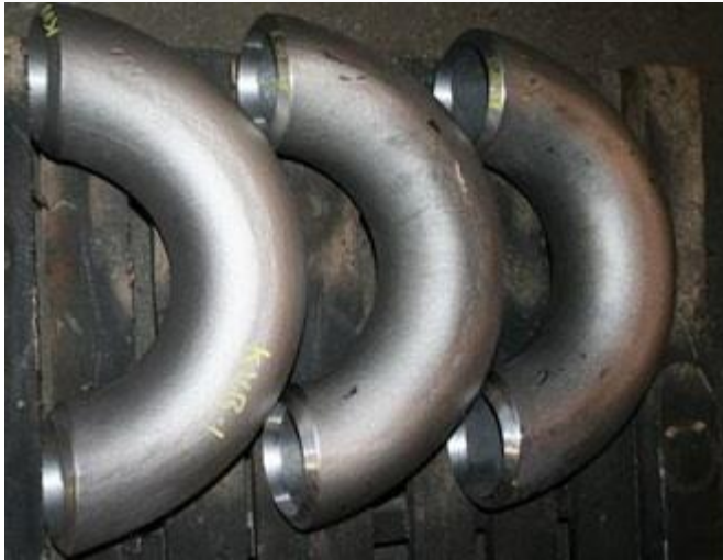
Stainless steel 316L, ASME B16.9 short radius(S/R) return, 180° 3" SCH80
